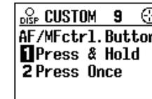
When in manual focus mode (MF), press once to select AF. Press again to return to MF mode.
