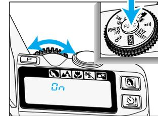
**2** While pressing the function button, turn the control dial until
