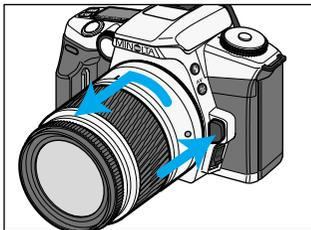
While pressing the lens release, turn the lens counter-clockwise until it stops. Carefully remove the lens.
