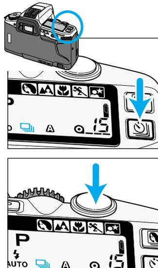
**1** Press the drive-mode button until appears on the data panel.
