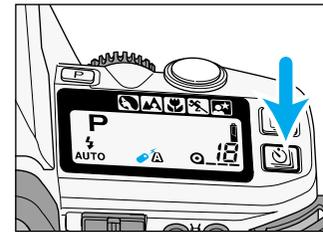
**1** Place the camera on a tripod. Press the drive-mode button until appears on the data panel.
