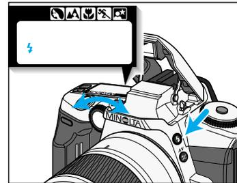
While pressing the flash-mode button
