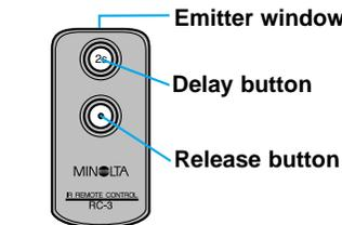
**3** Point the emitter window toward the remote-control receiver and press the release or the delay button.
