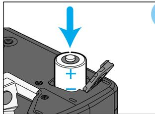
**2** Insert the batteries. Match the positive terminal mark inside the battery chamber-door with the positive end of the batteries.
