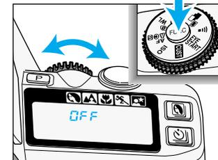
**2** While pressing the function button, turn the control dial to **OFF**.
