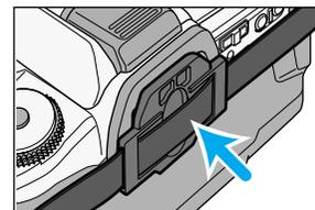
Firmly press the eyepiece cap of the strap into the eyepiece.
