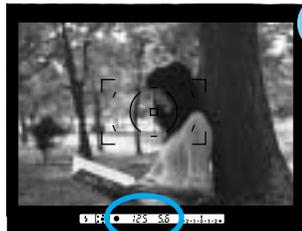
**1** Center your subject in the wide focus frame [ ], then press the shutter-release button partway down to lock the focus.
