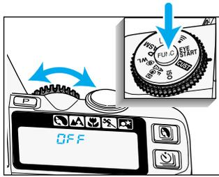
**2** While pressing the function button, turn the control dial until **OFF** appears on the data panel.
