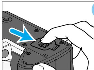
**1** Slide the battery-chamber release as shown, and open the door.
